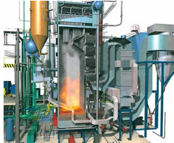
Rebuild of 17.5 MWth/4.3 MWe rice husk power plant in Chai Nat, Thailand 2000. Fortum Engineering Ltd.
